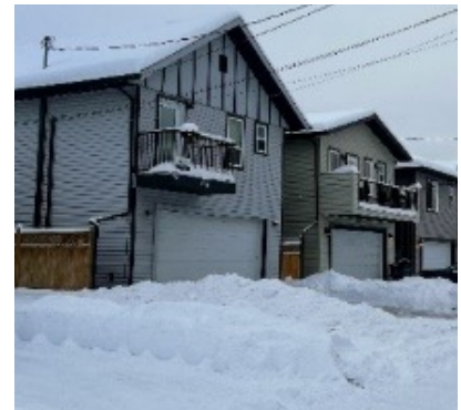
These infill homes have an approximately 7m setback that accommodates parking between the building and the lane and provides ample turning radii for vehicles entering and existing the garage.
